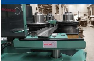
Hydraulic pulling unit for hard way beam rolling
